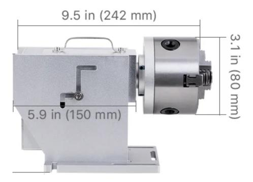
The DMS rotary accessory is used for radial marking of small to medium components. Designed to be plug-and-play with either of the Datamark ECO or XL laser systems. Driven by a NEMA 24 stepper motor and ability to adjust both height and angle the is the perfect choice for limited use or full production environments.
